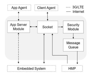
Fig. 3 The detailed block diagram of the middleware
